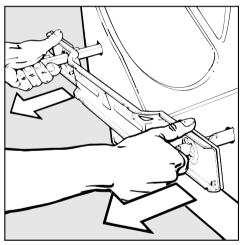
• Withdraw the two bars together with the support plate.
